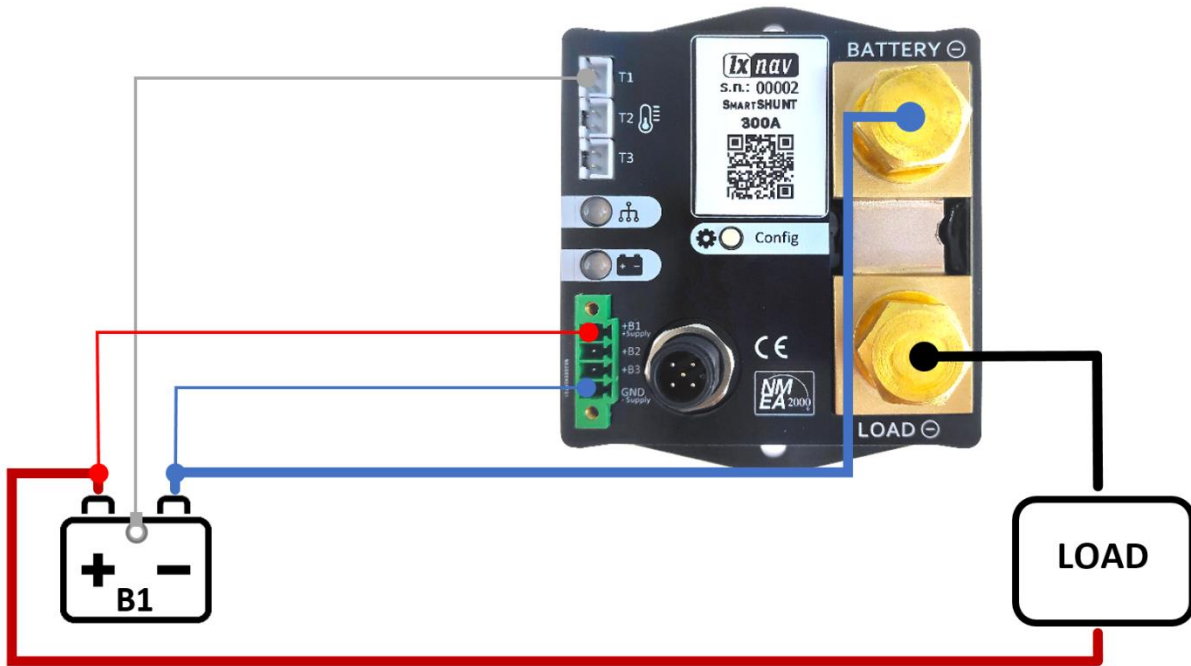
Figure 11: Wiring diagram for 1S Battery (e.g. 12V)
